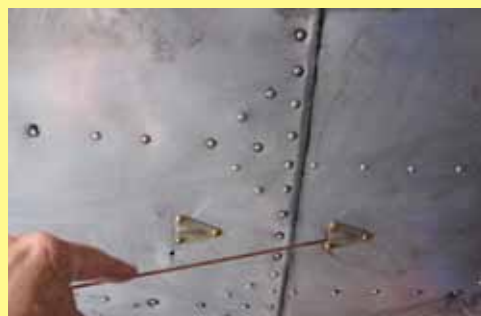
Water can get in where the window slides into the fuselage side. Drain holes allow water to drain out the bottom. It is mandatory to keep them unplugged, easily done with a piece of welding rod (below)
