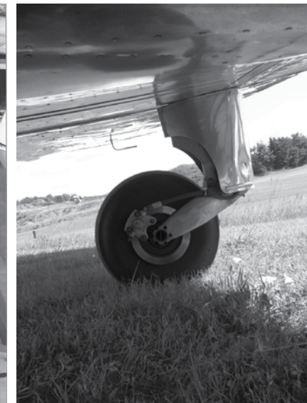
Left: the Ercoupe's unusual diagonal wing ladder eliminated the need for drag/antidrag bracing, shown here after priming and assembly. Centre, the main landing gear has a long travel trailing link suspended by an oleo with rubber pucks for suspension. Above right, the clean engine compartment with properly firesleeved fuel lines. Right, before and after pictures of the engine.
